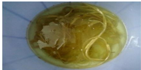
Figure 1 Treatment of Fiber in 2% NaOH solution
